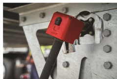
Landing Gear Lock Covers and locks the landing gear handle.
