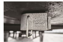
King Pin Lock Secures dropped trailer.
