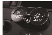
Air Cuff ® Lock Prevents truck and trailer brakes from being released.
