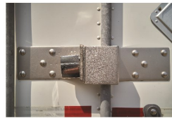
Trailer Door Hasp Lock Protects side or rear door of trailer.
